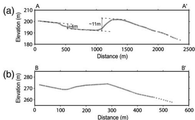
**Figure 6.** Topographic profiles across the Luyeh strand on the Lungtien and Yongan surfaces. Instrument uncertainties are at about the centimeter level and are too small to show at the plotted scale. (a) Topographic profile across the Luyeh fault on the Lungtien surface. Elevations were surveyed using a total station along a major road on the Lungtien surface. (b) Topographic profile across the Luyeh fault on the Yongan alluvial fan.
