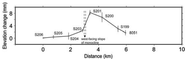
**Figure 5.** Leveling profile of the Lungtien surface across the Luyeh strand. The leveling route is shown in Figure 4b. The observation period is from April 2002 to April 2003. Elevation changes are referenced to site S206, located on the relatively stable Central Range block. Uncertainties are one standard deviation.
