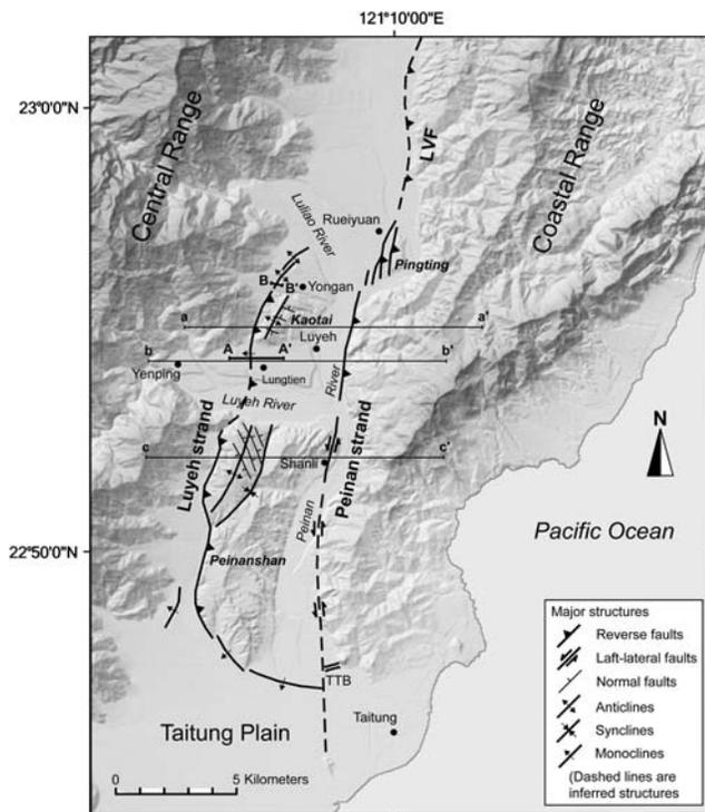
**Figure 3.** Active faults of the Luyeh area, modified from Shyu *et al.* (2008). South of Rueiyuan, deformation is accommodated by the Luyeh and Peinan strands of the Longitudinal Valley fault. In the northern Peinanshan, the anticline–syncline pair represents fault-related folding above the Luyeh fault. The locations of topographic profiles AA' and BB' (Fig. 4) and tectonic east–west cross sections aa', bb', and cc' (Figs. 8 and 10) are shown. The Taitung Bridge is indicated by TTb.
