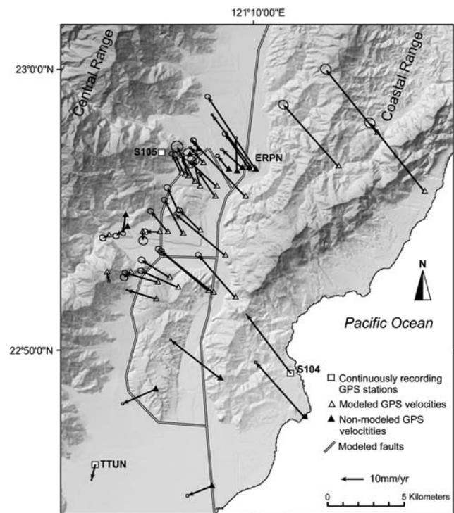
**Figure 7.** GPS velocity field with model faults. The open triangles are GPS velocities used as constraints. The filled triangles are velocities that were not used to constrain the model. The model relied primarily on GPS velocities around Yongan, Kaotai, Lungtien, and northern Peinanshan.
